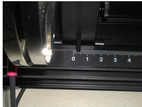
Figure 3: Detail photo of capacitor plate indicator foot
